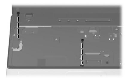
Where used: 2 screws that secure the top cover to the base enclosure (top)
